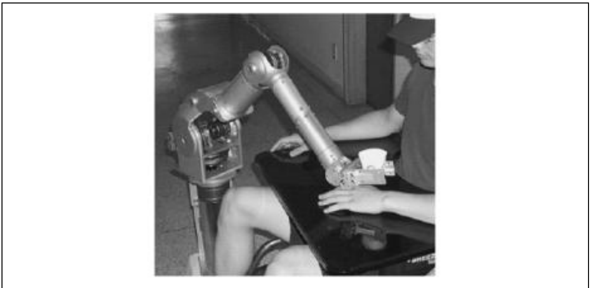
Figure 3 – KARES-II, the KAIST wheelchair-mounted robotic arm (11)
